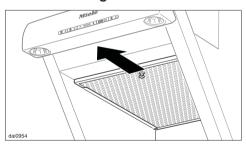
■ Pull the grease filter by the hand-hold forwards and out.
